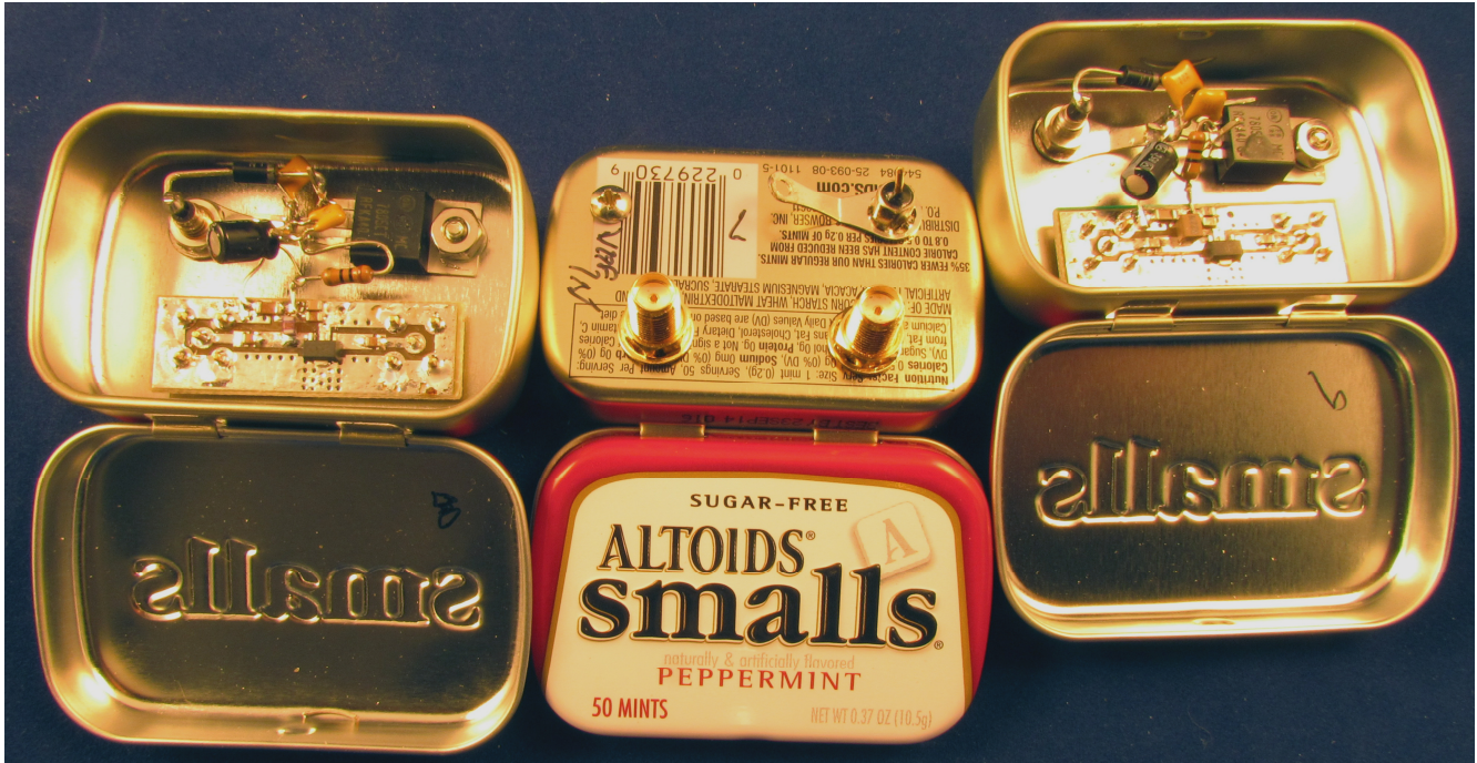
Figure 1- MMIC preamps in Altoids tins
