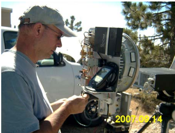
A view from the other side of the 79 GHz rig showing the Icom computer transceiver operating on 1296 IF with Palm for a small portable rig.
