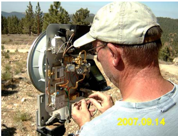
Gary, AD6FP on Frazer DM04ms doing the code the hard way with clip lead to Doug, K6JEY on Pinos DM04kt 15 km away with 79 GHz.
