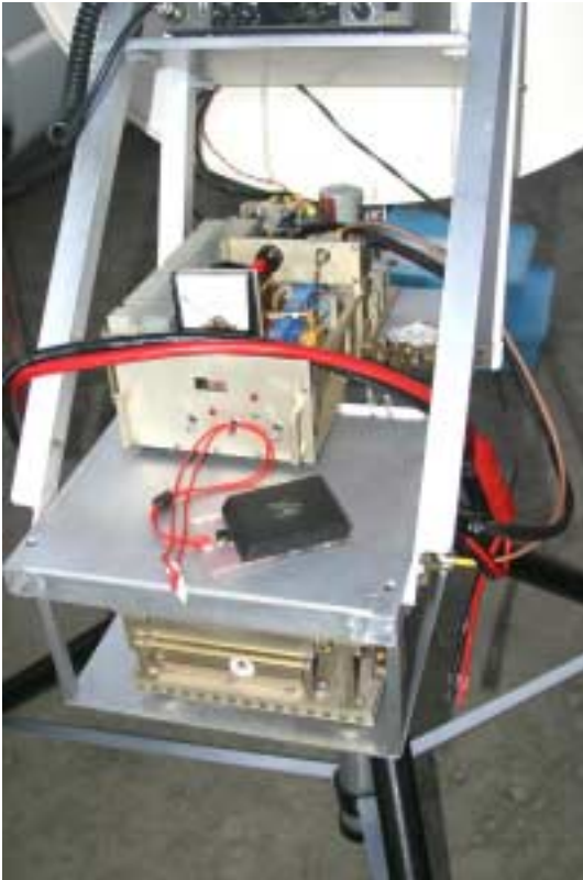
Chip, N6CA new model of 10 GHz rig with bigger power amplifier.
