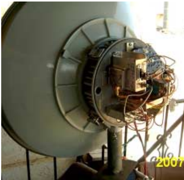
Pcom 24 GHz rig on the back of its 2 ft dish. The original feed is 3/8-inch hobby brass tube leading to a splash plate.
