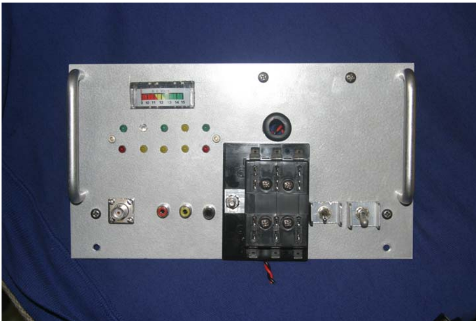
The front panel includes a battery charge meter, fuse block, IF interconnections and status indicators. Labels will be added later.
