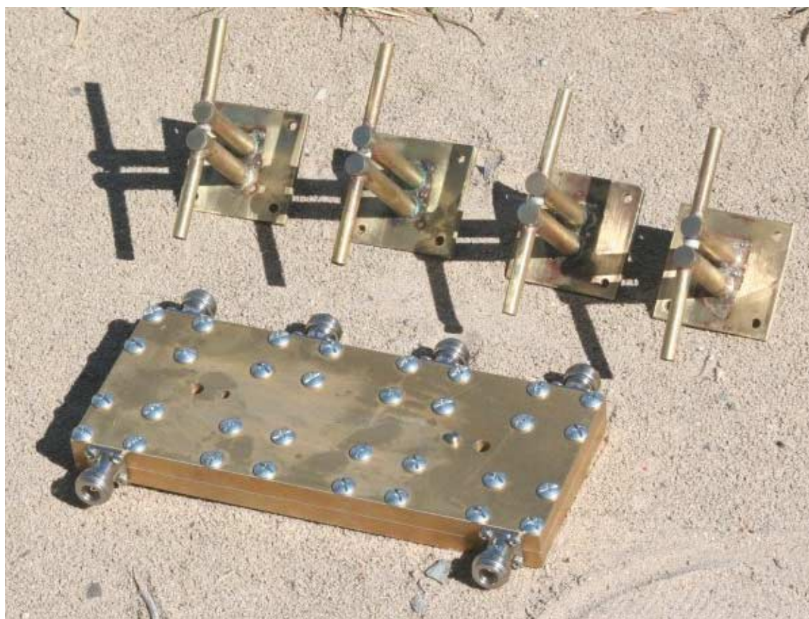
The 4 dipoles and hybrid built by Dick, K6HIJ to install at OVRO feed area so we can work 1296 MHz EME with right and left circular polarizations.
