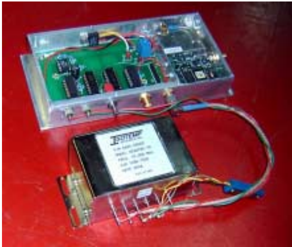
Dave, WA6CGR carried in his 10 MHz GPS referenced frequency standard that he picked up off pyrojoes ebay list. Joseph sells the kit boards and components along with the Jupiter GPS receiver. He also sells the OCXO.
