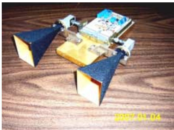
Juno KG6MQS 47 GHz rig with surface mount parts.
