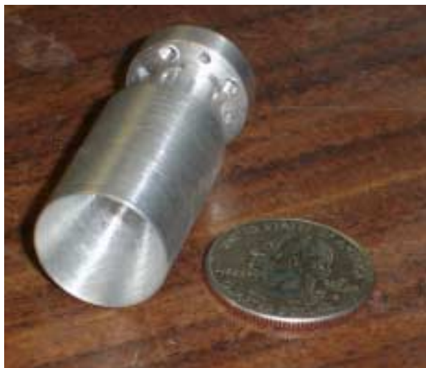
The 78 GHz horn built by Dick, K6HJJ.
