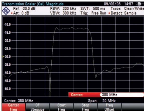
Scalar transmission measurement
