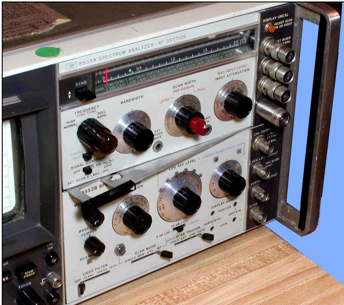
Release Lever Holding the Spectrum Analyzer Sections
