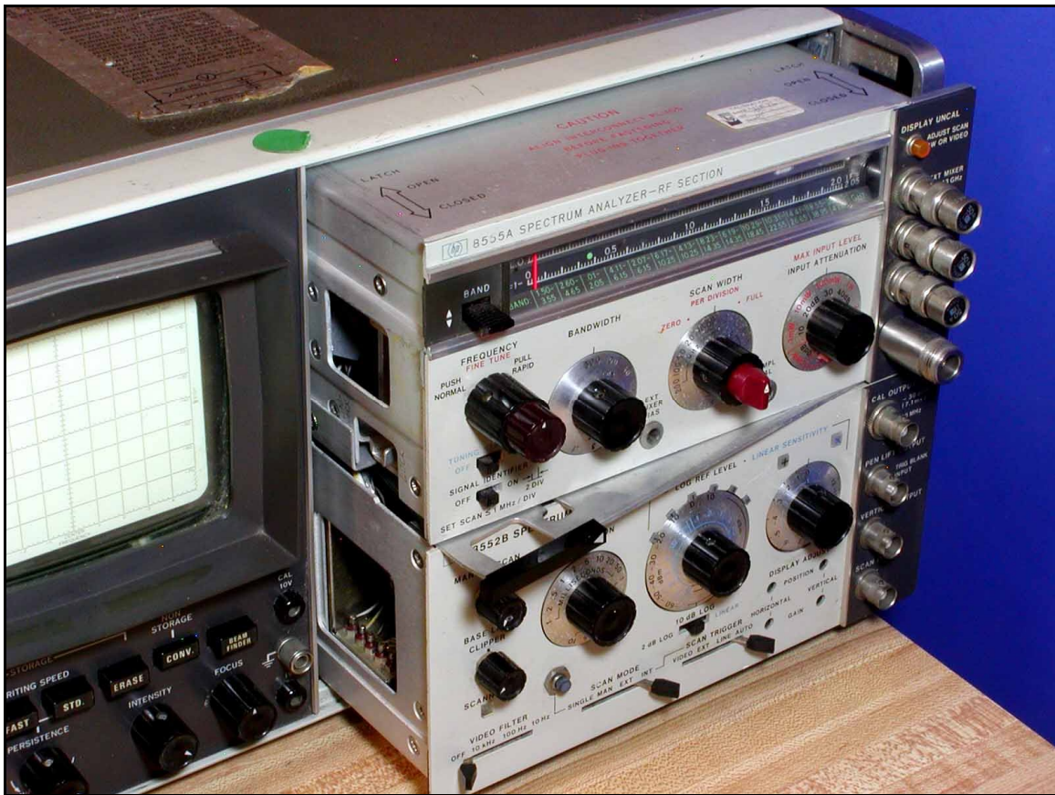
Pull Analyzer Straight Out of the Display Section
