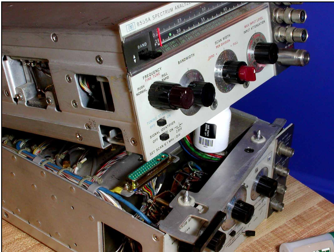
Lift the Front of the RF Section About 2 Inches to About the Position Shown, Then Slide It Backward To Separate It From The IF Section. (A Pill Bottle Is Used Here To Hold the RF Section for the Photo)
