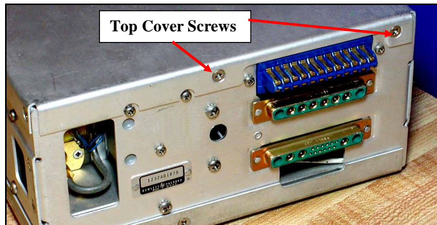
Rear of RF Section – Remove 2 Top Cover Screws
