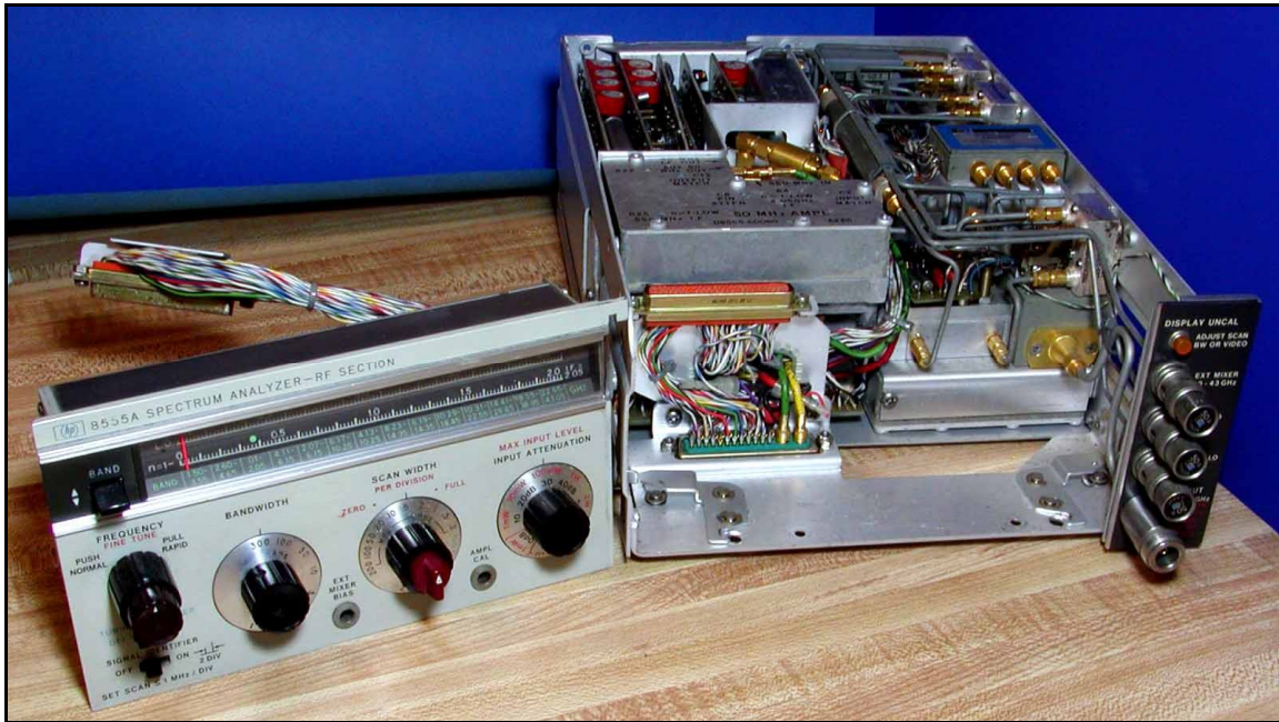
Front Panel Removed From HP-8555A RF Section
