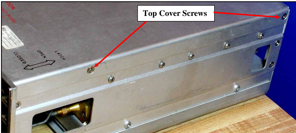
Right Side of RF Section – Remove 2 Top Cover Screws
