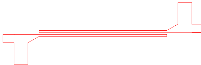
Figure 8 – Layout of Edge Coupled LO Filter
