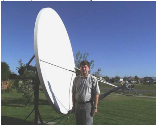
Figure 1 2.4 m Offset Reflector for 24/47 GHz
