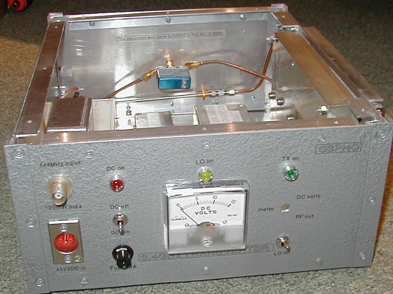
3.4GHz 14 watt transverter by G3PHO. March 2003
