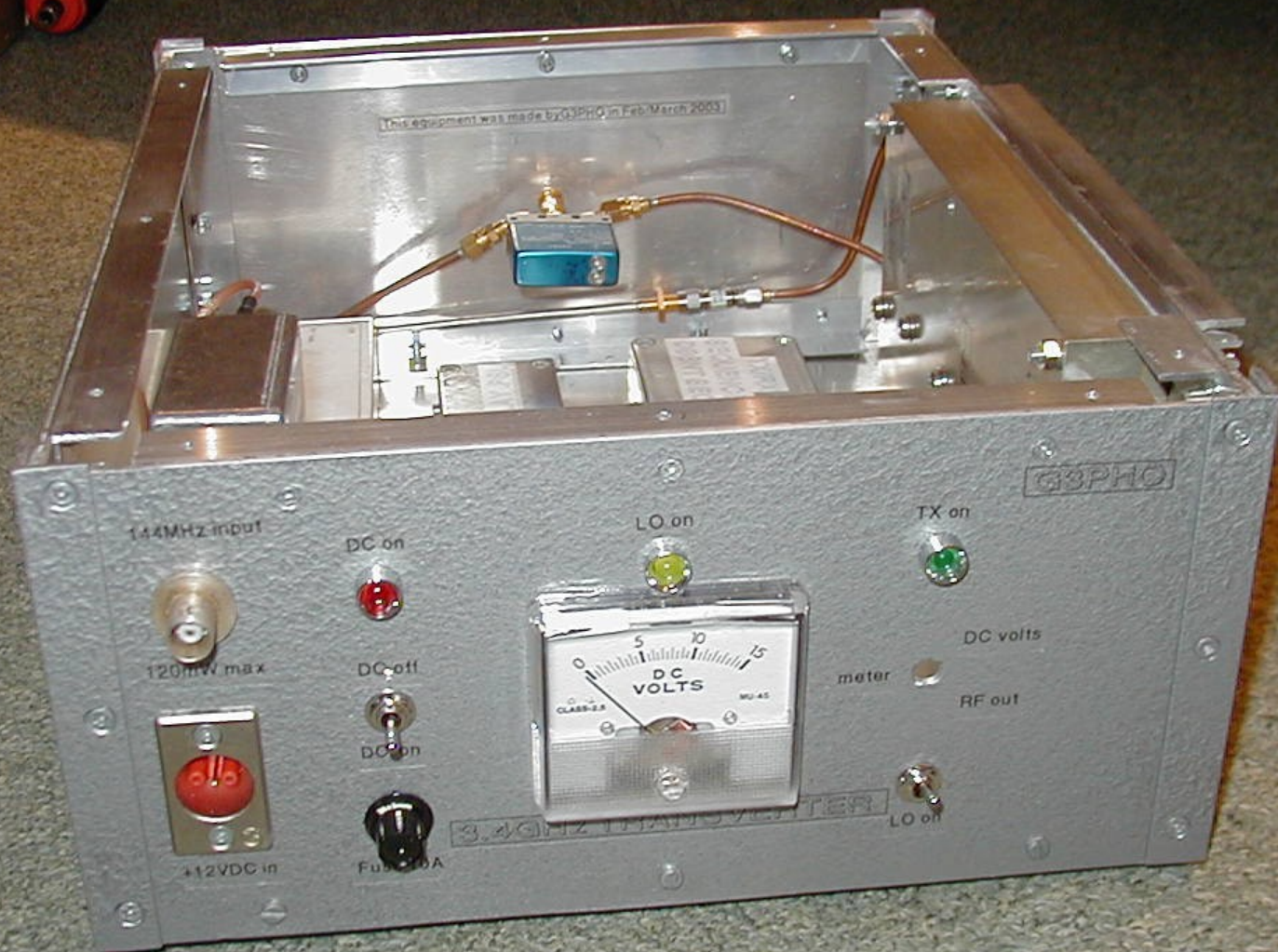
3.4GHz 14 watt transverter by G3PHO. March 2003
