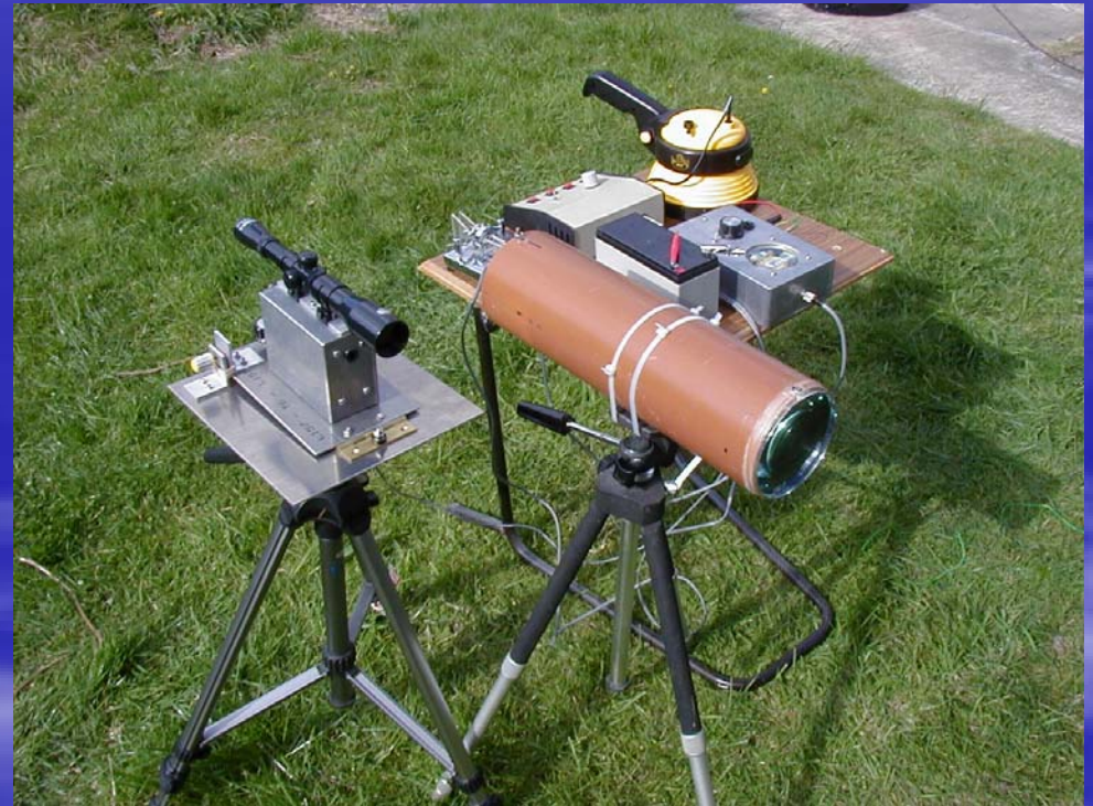
F/G0MRF/P's laser transmitter and receiver setup
