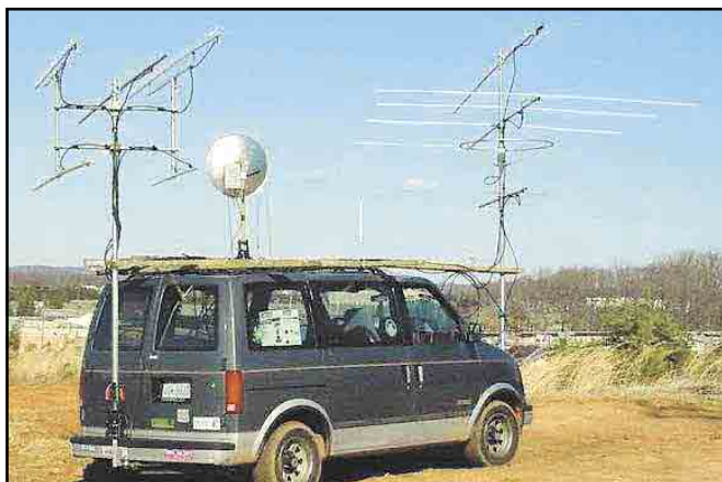
Microwave is often a part of VHF/UHF contesting. This “rover” station by W3IY was used in the 2002 June VHF QSO Party.
