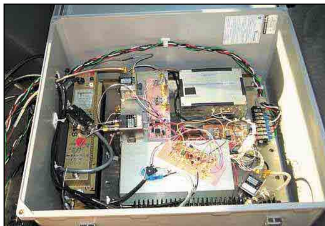
N1MU crafted this homebrew 10-GHz transverter.
