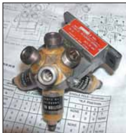
Figure 3—This photo shows a surplus Transco brand four-port N-type relay.
