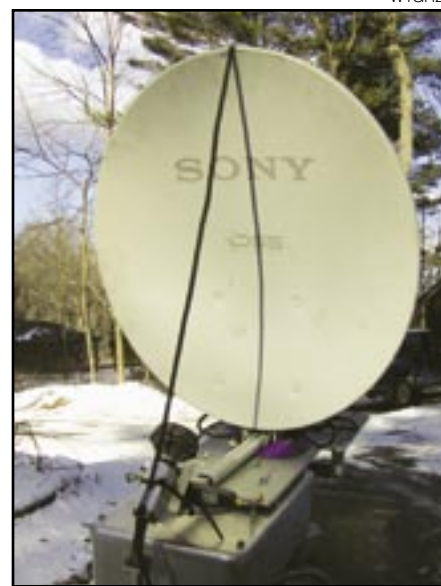
Figure 2 — String shadow on dish lines up with sun.
