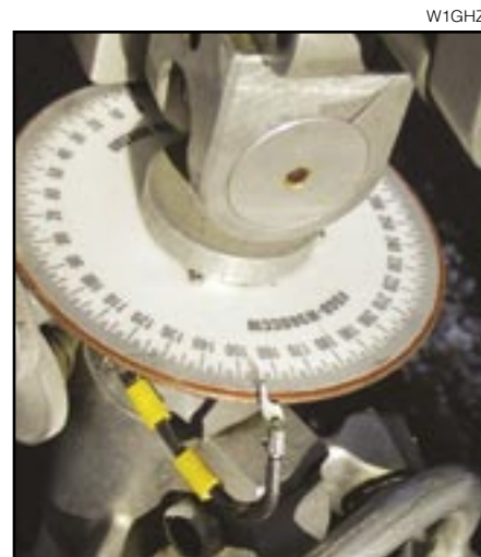
Figure 3 — Azimuth setting circle or compass rose on tripod.
