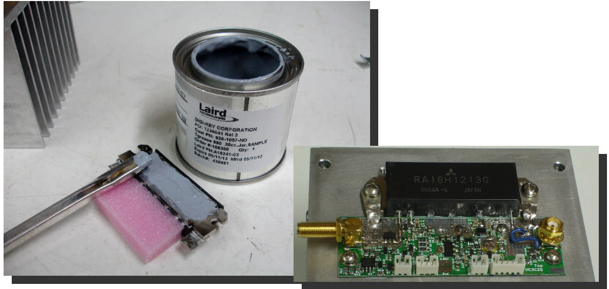
Fig. 9 RF PA & PCB Mounted to Heat Sink
