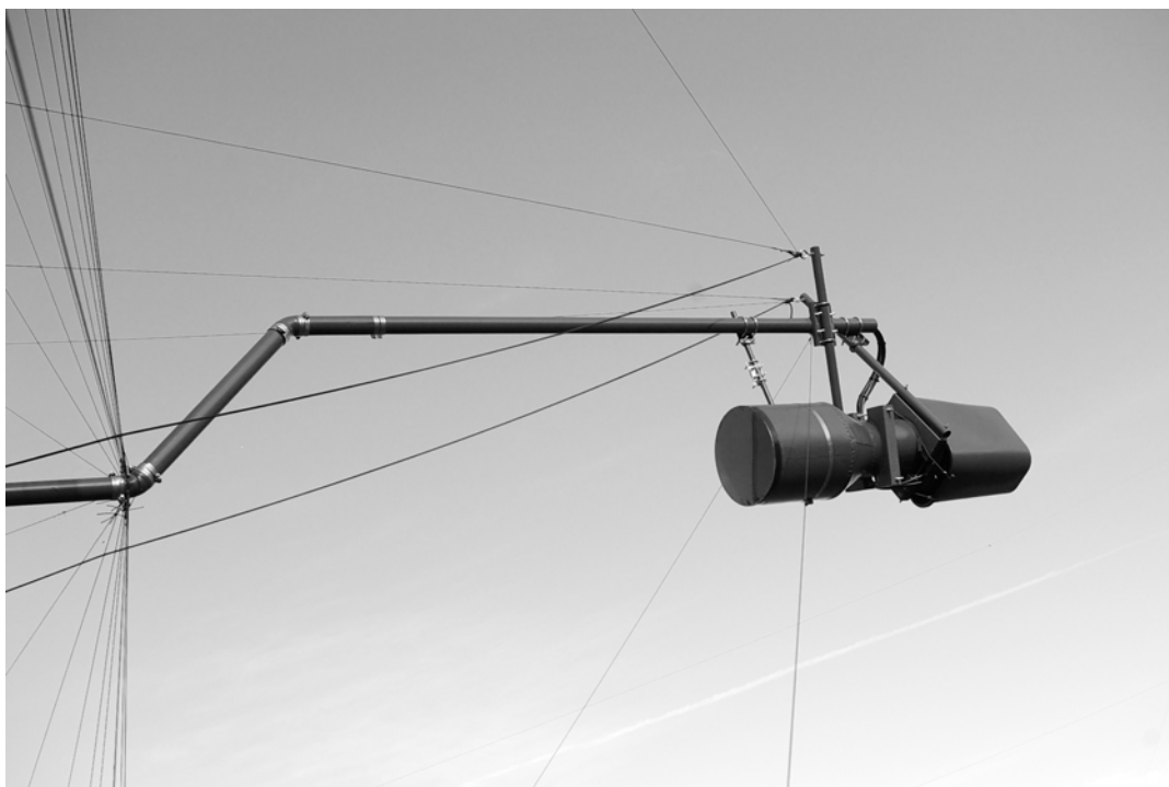
Fig. 13 – View of the feedhorn and support structure.
