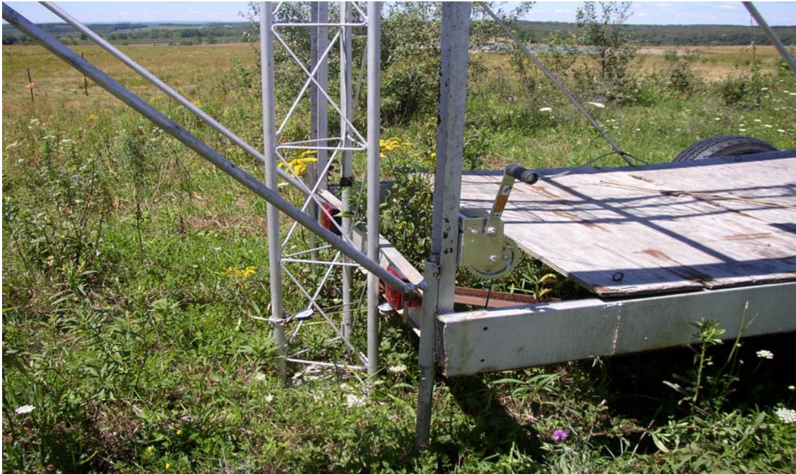
Winch for tilt-up tower on 6 meter trailer
