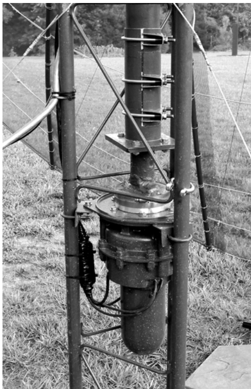
Fig. 3 – Prop pitch motor used for the azimuth movement.
