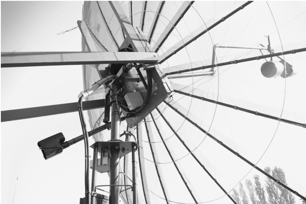
Fig. 5 – Hub and elevation actuator. The white box is the optical elevation sensor.
