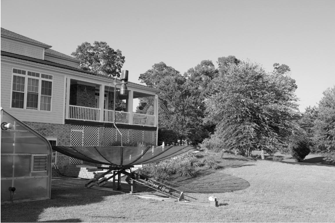
Fig. 1 – The antenna is kept close to the ground at 90 degree elevation when not in use. Note the support structure to relief the winch.
