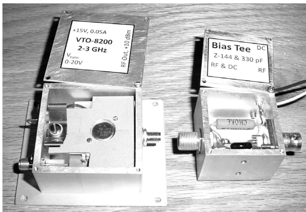
Photo D: Completed Enclosures with Internal Circuitry and Ready for Use
