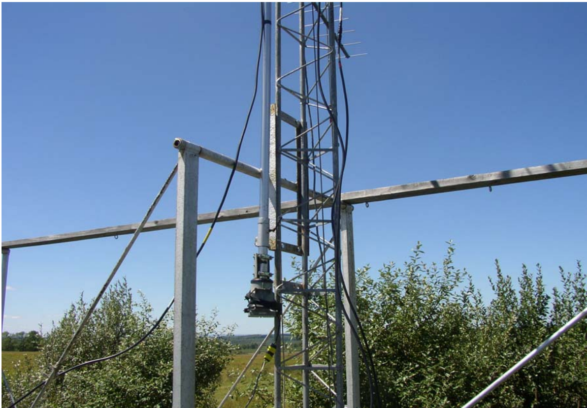
Pivot point for the tower on 432 trailer
