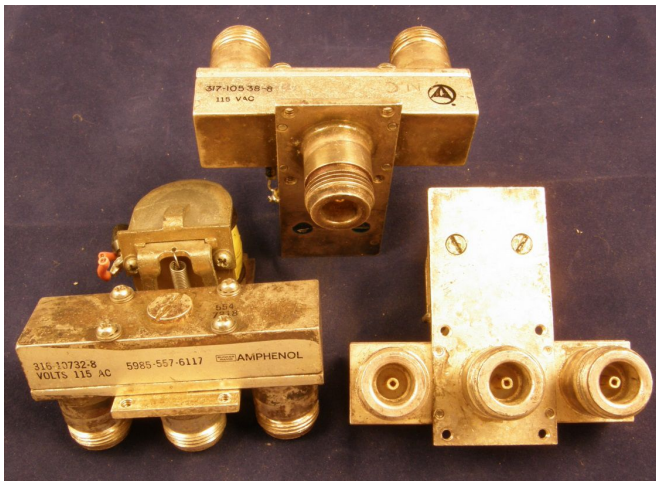
Figure 1 – Coax relays with marginal isolation at 1296 MHz
