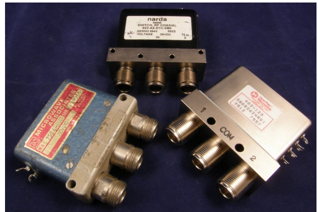
Figure 2 – Coax relays with good isolation at 1296 MHz
