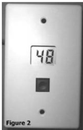
The indicator unit, in Figure 2, is a simple two-digit readout with a pushbutton which turns it on for a minute or so. It may be powered by an internal 9-volt battery or an external 12 volt supply. A four-wire cable connects the two units together; the cable supplied might be long enough for an RV, but I added some cheap rotor cable to reach up the tower.
