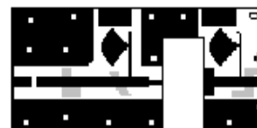
Figure 4: Circuit board after tuning. Stubs shown in grey.
