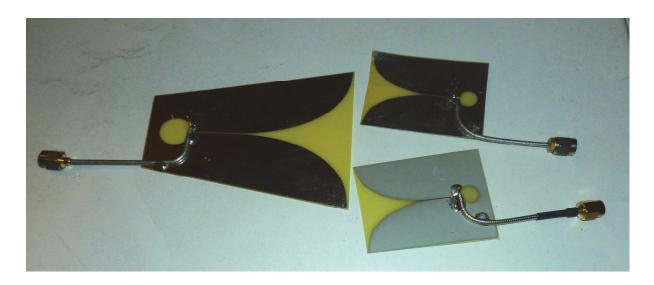
This is a project I plan to expand in the coming weeks. Here a Vivaldi antenna is used with a bit of coax and a microwave diode to form an external mixer for a spectrum analyzer.
