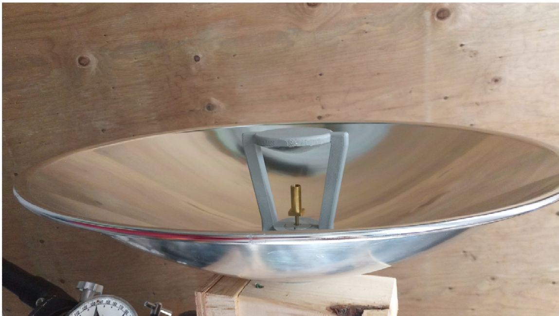
Figure 13 – 24 inch Cassegrain Antenna with Large W2IMU feedhorn for 47 GHz from Figure 5 by VE2UG
