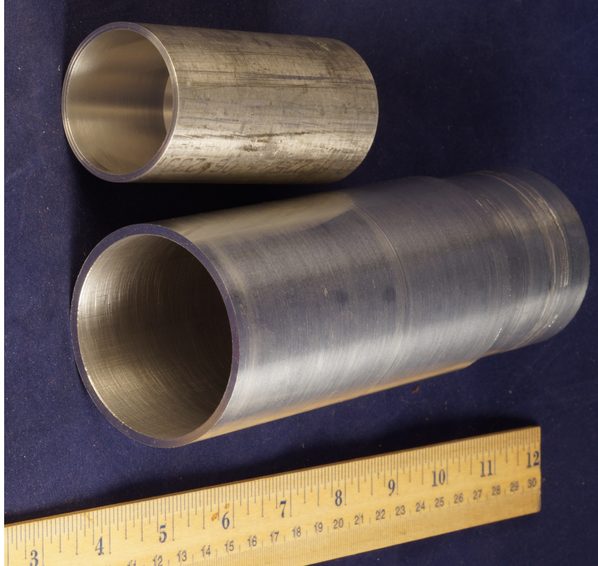
Figure 11 – Large ( 1.88\lambda ) and Small ( 1.31\lambda ) W2IMU Feedhorns for 10 GHz
